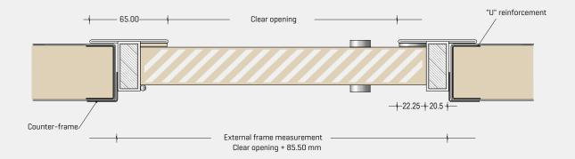
External frame measurement= Clear opening + 86 mm Cavity to be opened in the panel= external frame measurement + 10 mm
